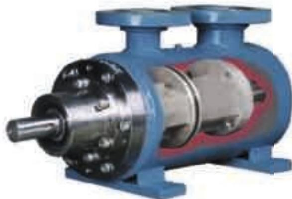
This range is designed for medium pressure applications on clean liquids. It is produced as a cartridge design. The cartridge has an aluminium alloy or SG iron construction and features mechanical seal and optional integral relief valve as standard. The cartridge doubles as a renewable sleeve and can be inserted into a fabricated steel casing to meet the requirements of API specifications. Custom casing designs can be accommodated to meet client dimensions and specifications.
