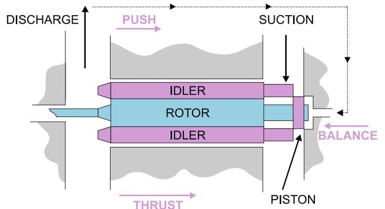
Push - Balance = Small residual thrust to avoid shuttling  $\longleftrightarrow$  under varying loads
